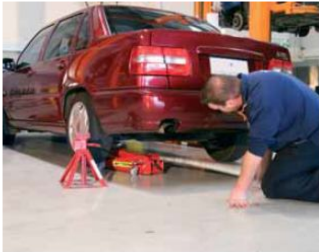
Figure 1.3b: Low risk workshop activity: Trolley jack and axle stands must be used at all times.
