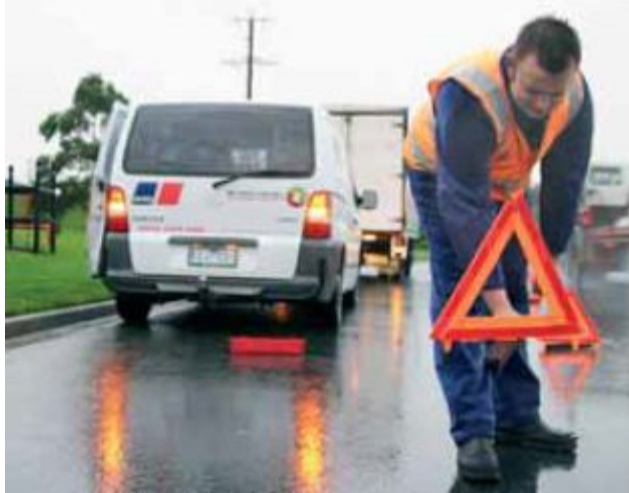
Figure 1.2a: Low risk workshop: Visible warning signs for approaching drivers
